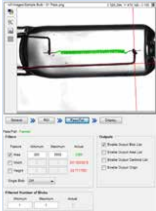
Tool parameter setup with graphical controls
